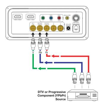
Figure 3-12. Progressive Component Video Connections
